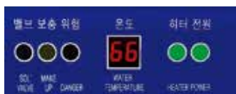
Digital display (Displays operation status and error code)
